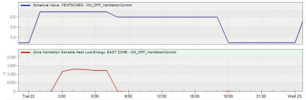
Figure 7: The ventilation rate and the overall loss energy
