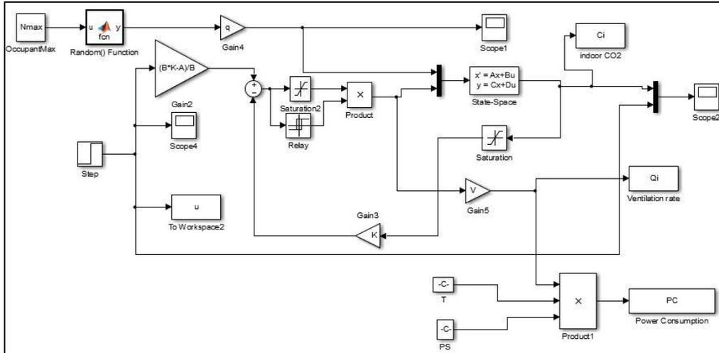
Figure 3: The State feedback control under Simulink
